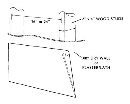
The center of the stud can be located by probing the wall with a small nail to find the edges of the stud and then placing a mark half way between the edges. The center of any adjacent studs will be 16" or 24" from this mark.
